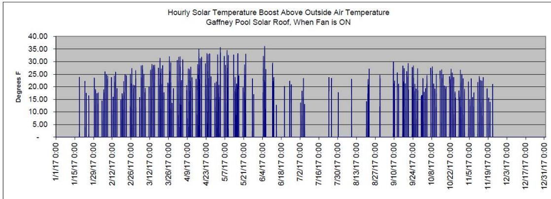
The annual solar energy delivery to the outdoor air intake is calculated by the multiplying solar air mass flow (#/hr), by the temperature rise above outdoor air temperature, by the specific heat of air, (.24BTU/#/deg-F), counting each ON hour. Heat energy delivery varied from 112,000 BTU/hr with a 36.9F solar air temperature rise down to 12,600 BTU/hr just before shutting OFF at 4F above outside air temperature.
