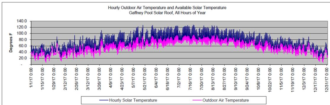
The actual hours per year when the solar air would be used was determined by accounting for the pool operating hours (44 open hours/168 hour week) and the constraint that the solar air would not be used when the outdoor air was above 75F, when cooling
