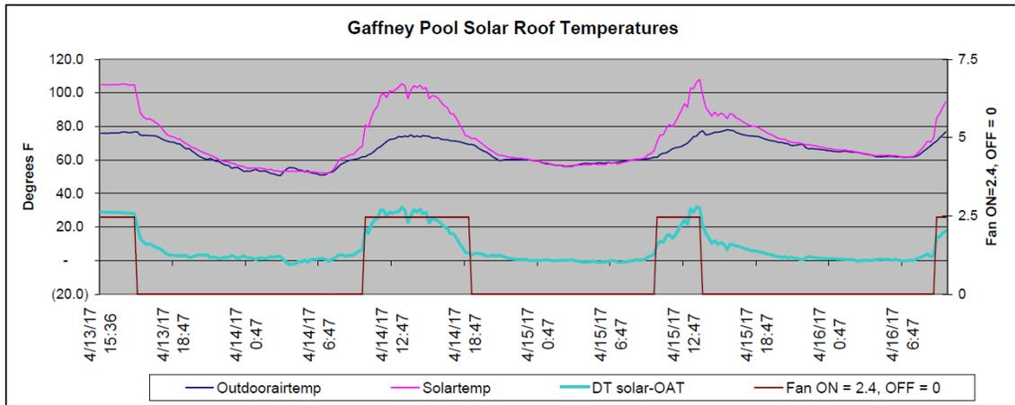
Using the monitored data, American Solar was able to confirm that the pool roof solar air temperature could be modeled using the same predictive algorithm developed for the earlier gym roof project, when accounting for the different roof slopes.
