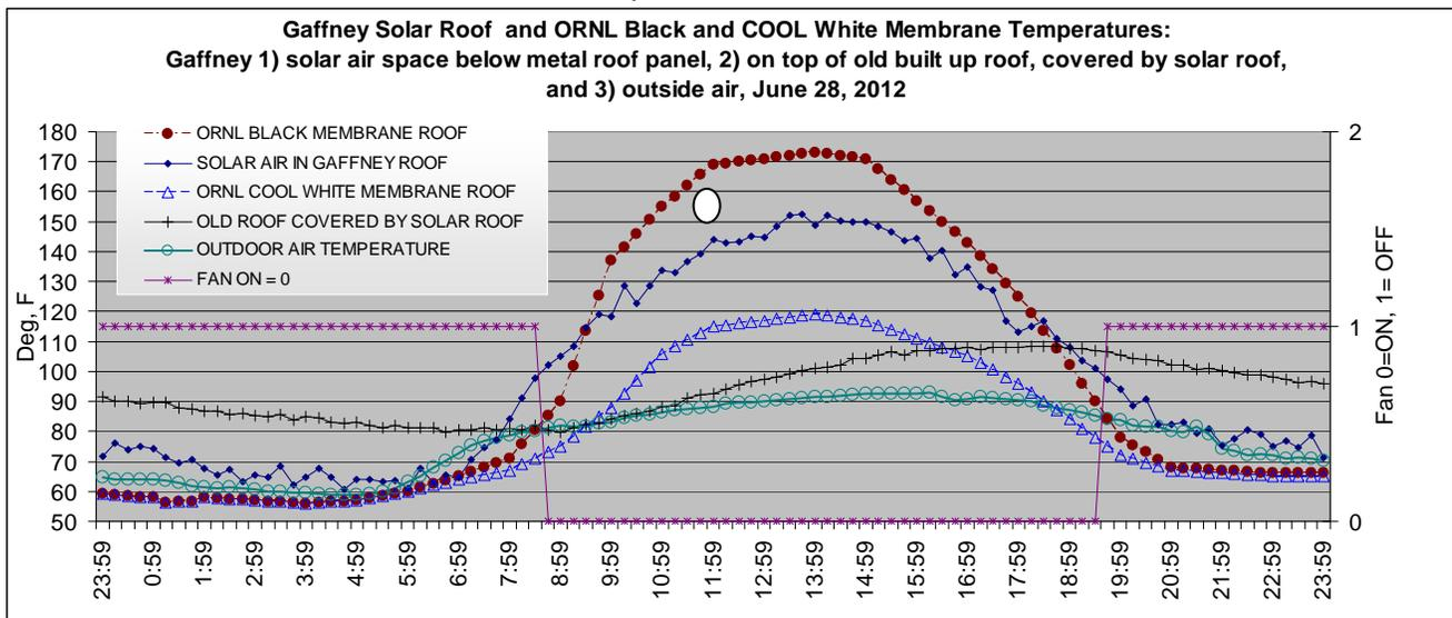
Figure 4 Temperatures of a ‘Cool’ Roof and Built up Roof Covered by the Solar Roof
