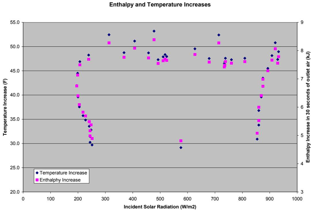
Figure 4: Enthalpy and Temperature Increases in Air at Low Flow with No Glazing
