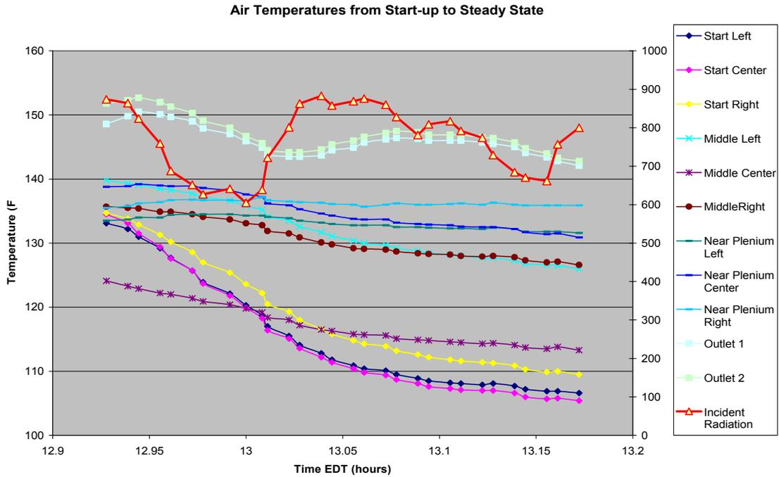
Figure 1: Air Temperatures from Start-Up to Steady State on July 10th
