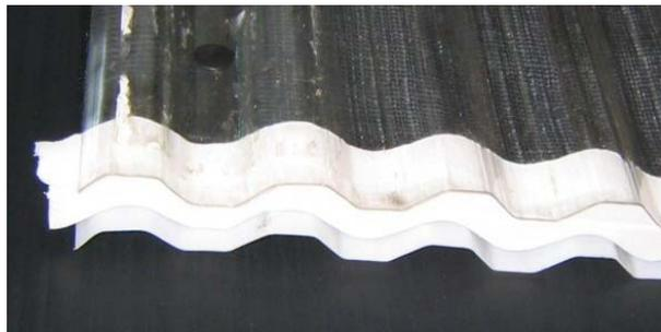
a lack of air plenum design or materials these collectors were not performance tested. The two collectors are approximately 32 square feet of GTP.
