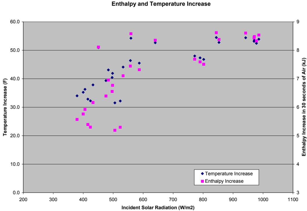
Figure 6: Enthalpy and Temperature Increases in Air at Low Flow with Glazing
