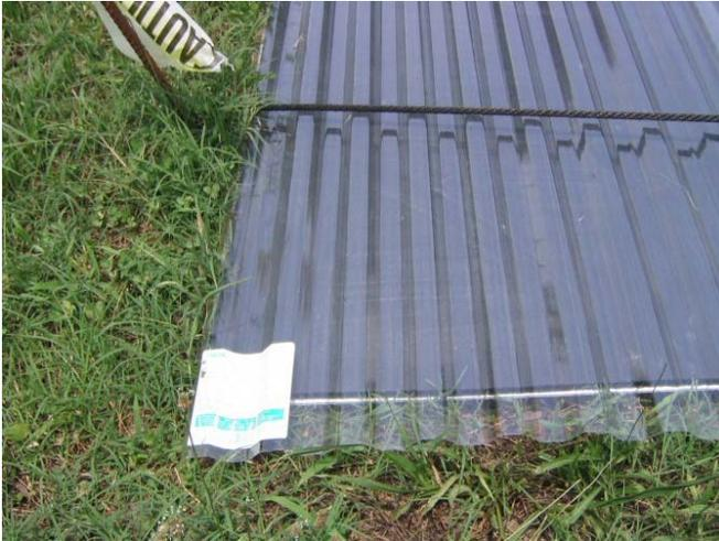
During some tests glazing was added to the top of the TFP in an effort to increase performance. Glazing material was off-the-shelf clear corrugated polymer panels laid on top of the TFP collector. This same glazing material was used to construct the second variety of low cost American Solar air heating panel, known as a glazed transpired panel (GTP).
