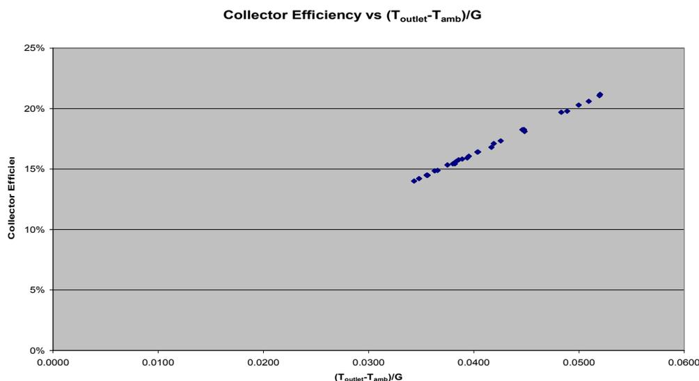
Figure 3: Collector Efficiency vs.  $T_{\text{outlet}} - T_{\text{amb}}/G$
