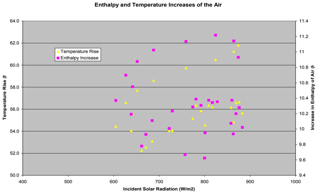
Figure 2: Enthalpy and Temperature Increases of Air Through Collector on July 10<sup>th</sup>
