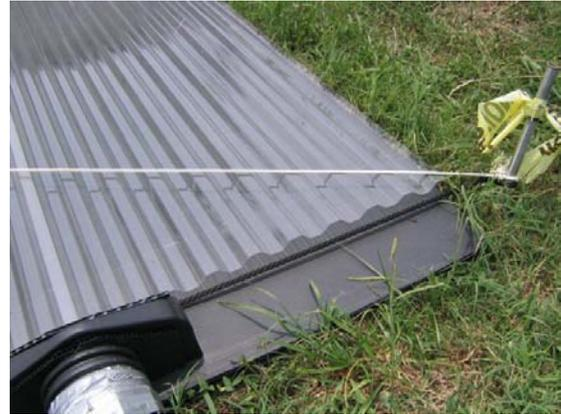
**System Efficiency (low angle): 19.6%** at an incident angle of 18.7° which was the average efficiency over 20 minutes under clear skies from 2:25 to 2:45 pm on Sunday July 10<sup>th</sup>. This region was chosen for the relatively stable incident solar radiation, stable output energy, and therefore stable efficiency.
