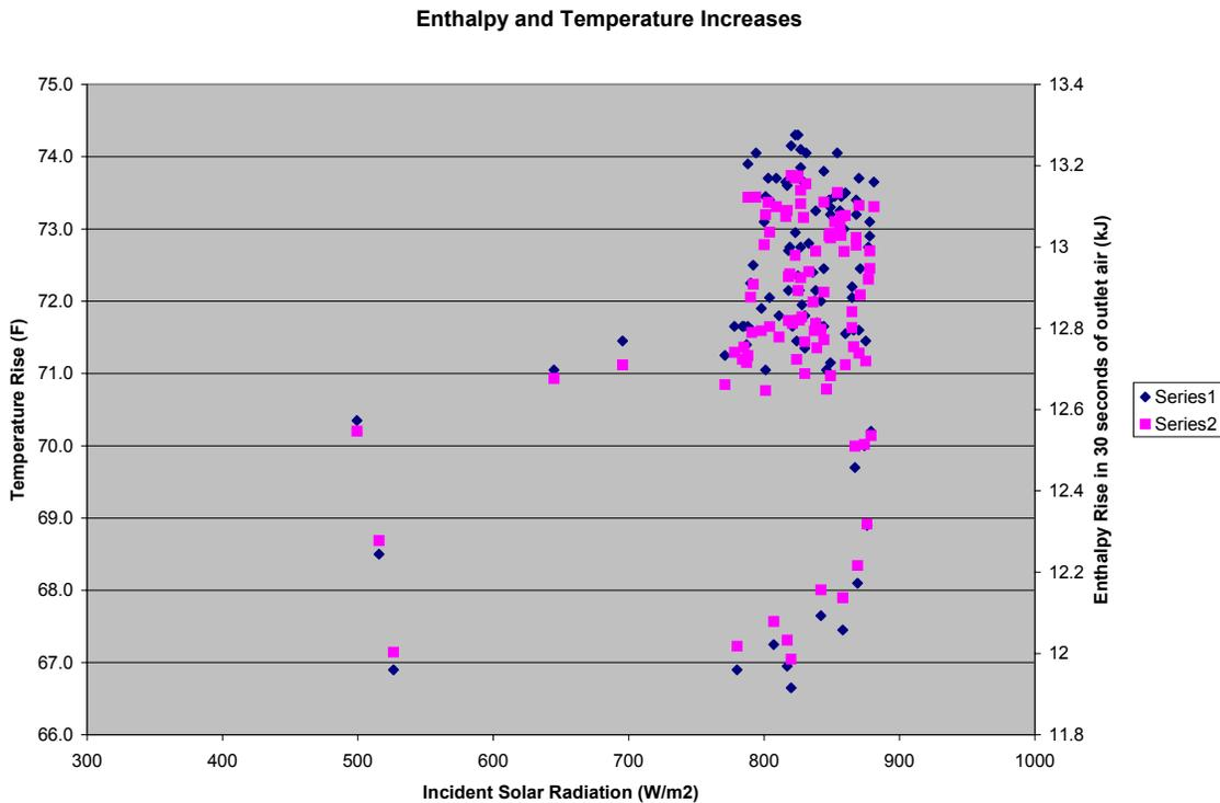
Figure 5: Enthalpy and Temperature Increases in Air at Full Flow with Glazing
