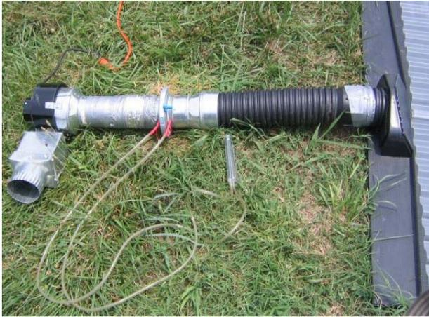
The Iris Damper not only allowed for airflow measurements to be made by measuring the static pressure difference before and after the iris, but it also functioned as a simple and repeatable way to adjust the airflow through the collector. Unfortunately with the large flow resistance of the collector, even large adjustments to the size of the damper opening had only moderate effects on the flow rate through the collector. With the fan connected to the collector and the
